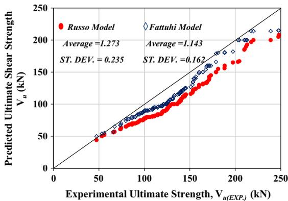
**Fig. 7** Comparison of the ultimate shear strength predictions using STM of Russo [17] and Fattuhi [3] with the experimental results
