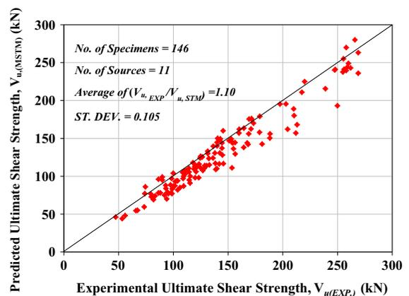
**Fig. 5** Comparison of the ultimate shear strength predictions using the proposed STM [14] and the experimental results
