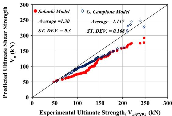
**Fig. 8** Comparison of the ultimate shear strength predictions using STM of Solanki [18] and G. Campione [19] with the experimental results
