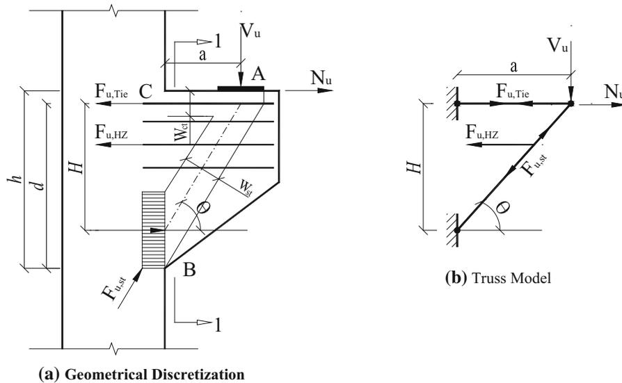
**Fig. 1** Elements of the strut and tie model of SFRC corbel
