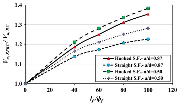
**Fig. 10** Effect of fiber aspect ratio ( $l_f/\phi_f$ ) on the shear strength predictions
