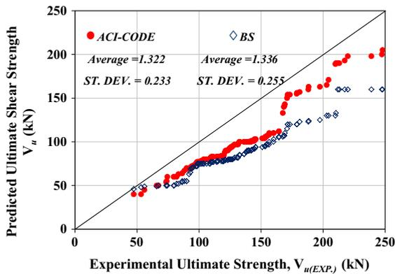
**Fig. 6** Comparison of the ultimate shear strength predictions using STM of ACI code [15] and BS [16] with the experimental results
