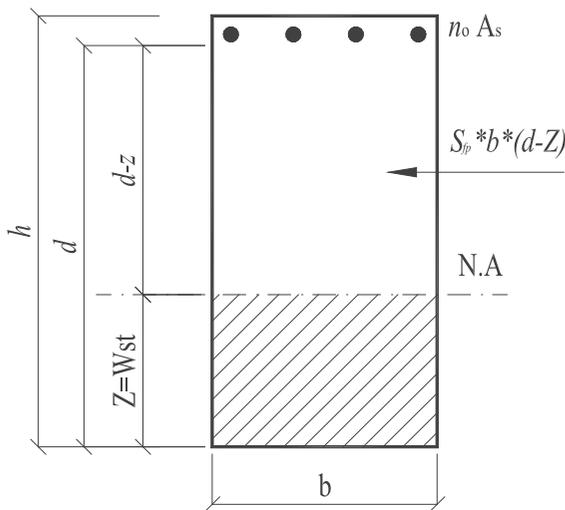
**Fig. 2** Illustrative sketch for the depth of compression and tension zones
