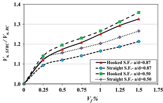
**Fig. 9** Effect of fiber volume ( $V_f$ ) on the shear strength predictions
