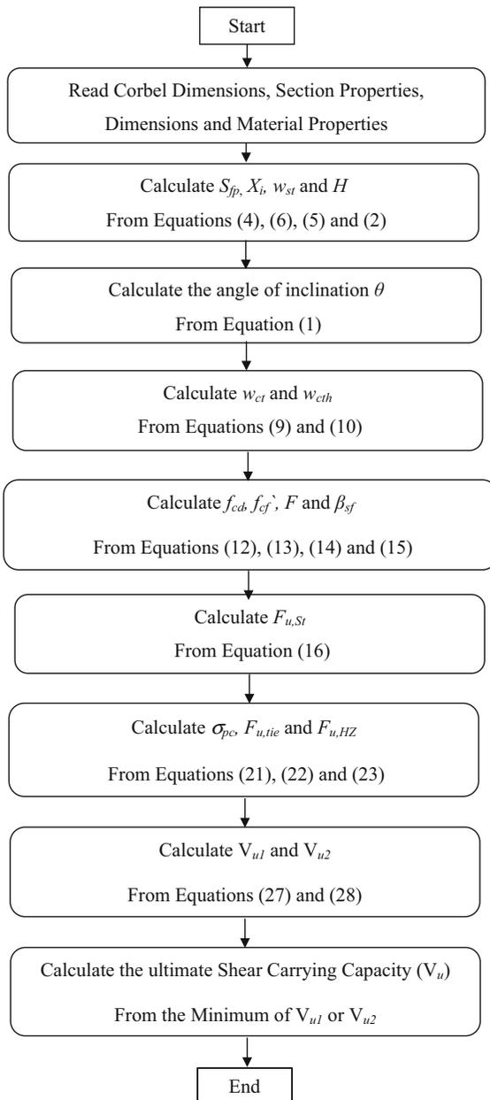
**Fig. 4** Implementation flow chart for the ultimate shear strength of SFR corbels
