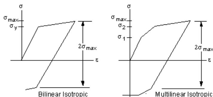
Fig. 1 Multilinear and bilinear stress-strain curves [4].
