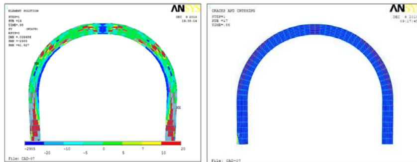
Figure 6: Unstrengthened vault stresses ( $\times 10^{-2}$  MPa) and crack pattern.
