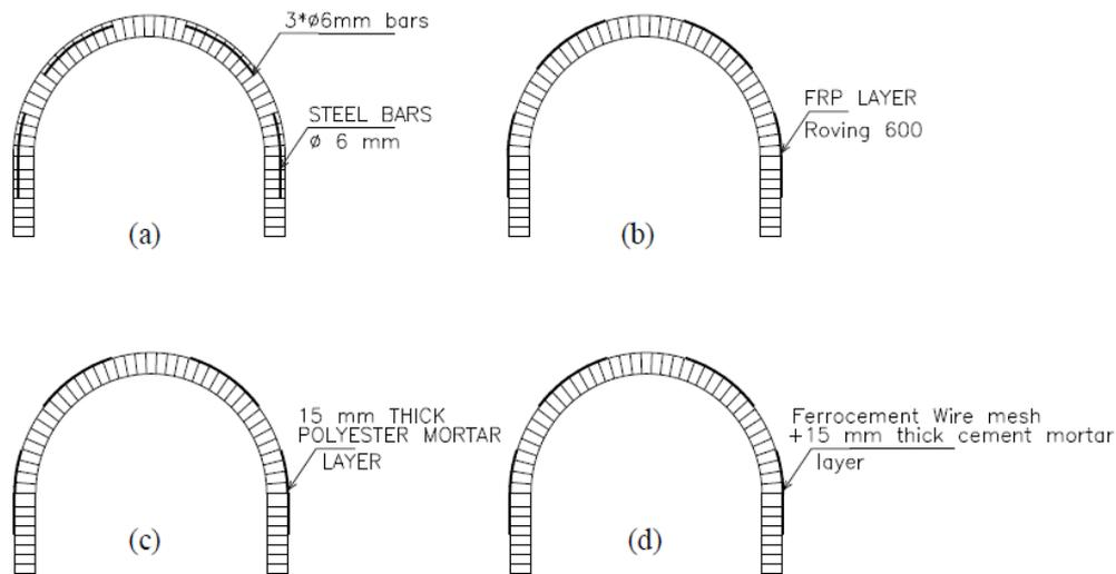
Figure 3: Strengthening techniques for the masonry vaults, a) Steel reinforcement, b) FRP sheets, c) external polyester mortar layer, d) Ferro-cement wire mesh [5].
