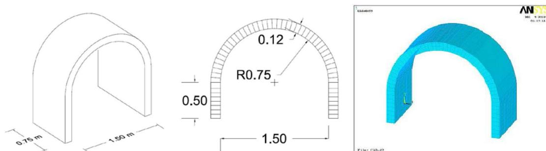
Figure 2: Dimensions and numerical model of the unstrengthened vault.
