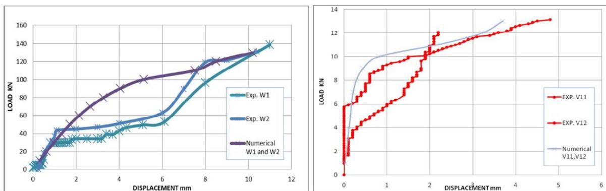
Figure 5: Load displacement curve for unstrengthened vaults and vaults strengthened by ferro-cement wire mesh
