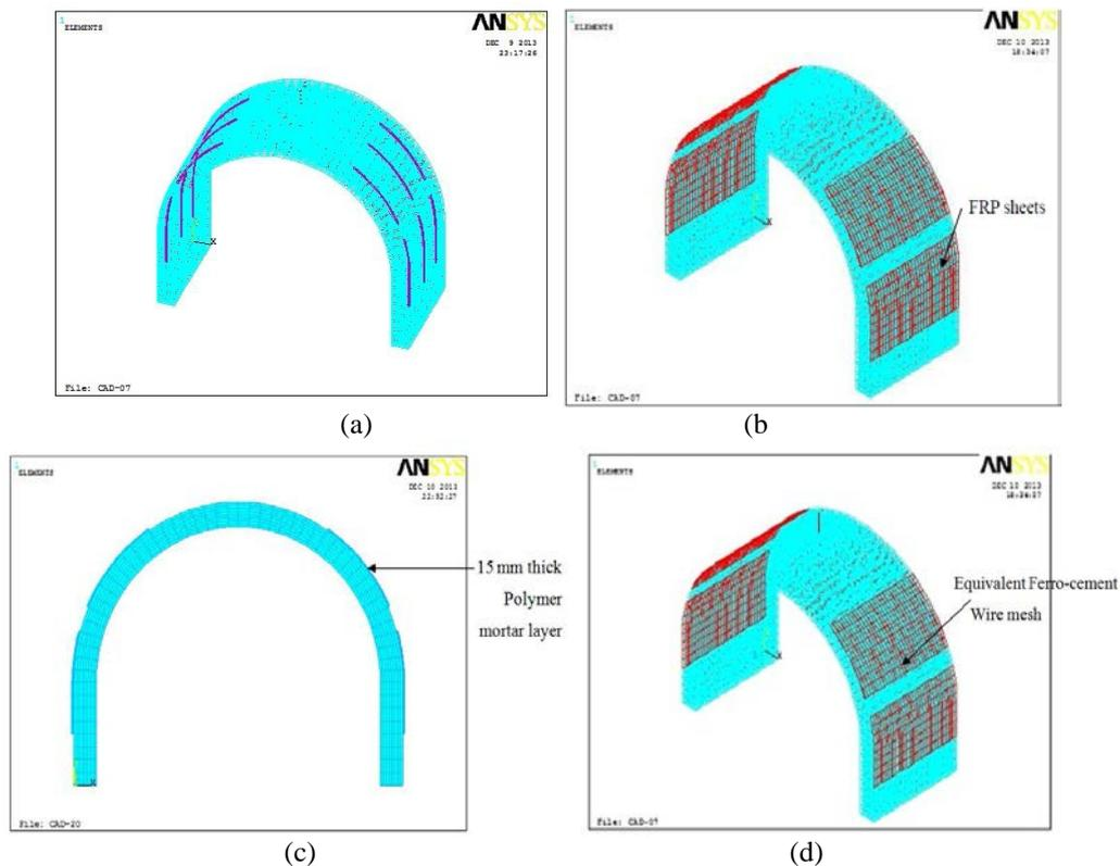
Figure 4: Finite element mesh of the strengthened masonry vaults a) Steel reinforcement, b) FRP sheets, c) external polyester mortar layer, d) Ferro-cement wire mesh [5].
