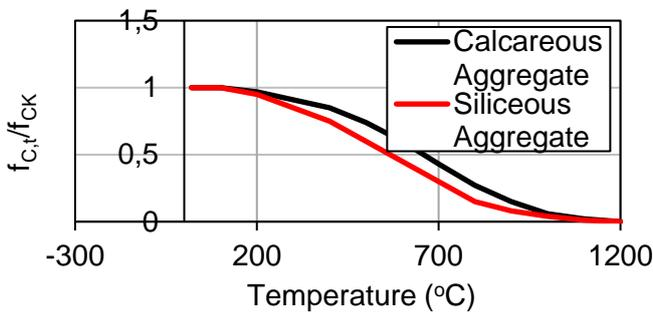
Fig. 9 - Variation of compressive strength of concrete with temperature [9]
