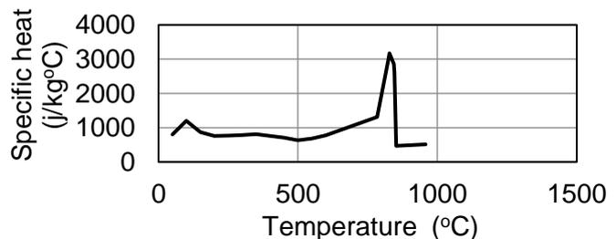
Fig. 21 - Specific heat of carbonate aggregate concrete [17]
