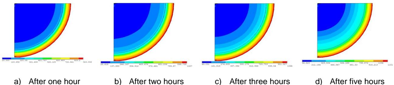
Fig. 25 - Column (1): Numerically predicted temperature distribution in the column cross-section
