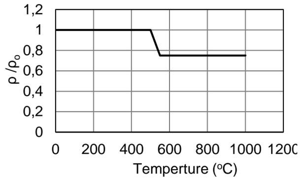
Fig. 2 - Variation of density of FRP with temperature [11]
