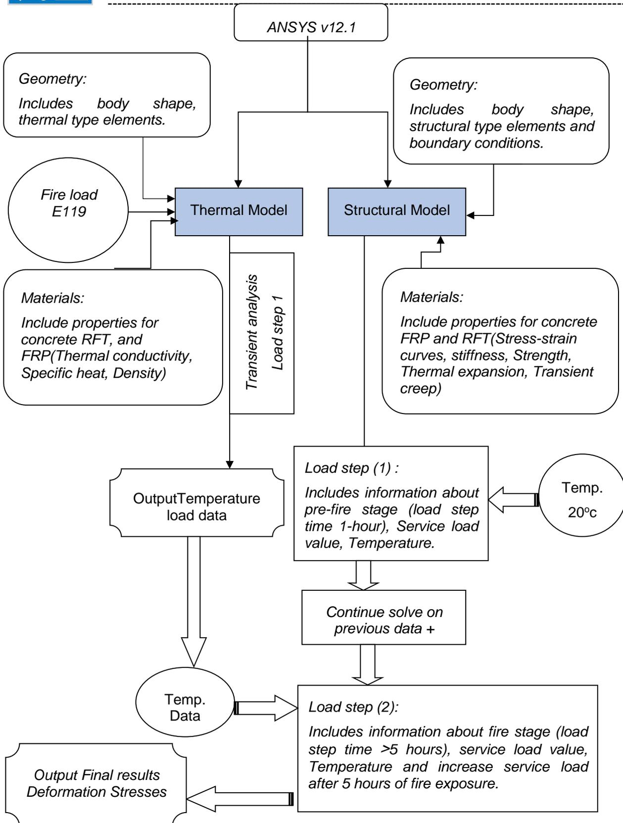
Figure 22: Schematic modeling methodology for RC columns strengthened with FRP
