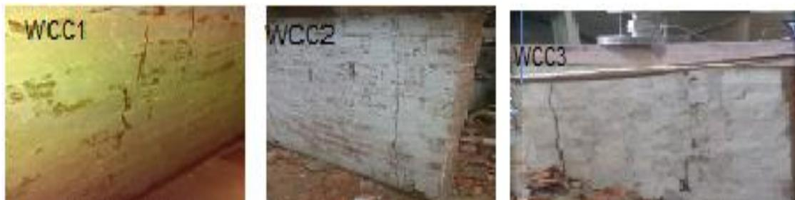
Fig 5. Failure mode of closed control wall WCC
