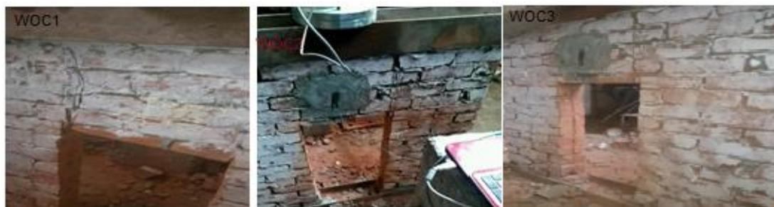
Fig 6. Failure mode of control walls with openings WOC
