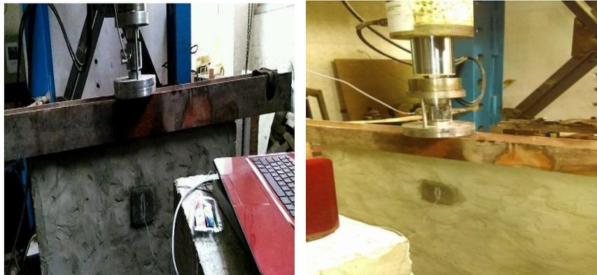
**Fig. 4: Test setup for loading and displacement measurement**
