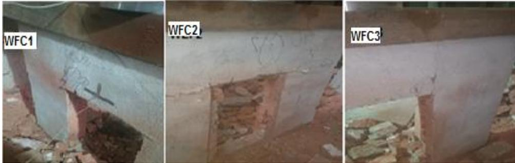
**Fig. 9: Failure mode for walls strengthened with ferro-cement layer**
