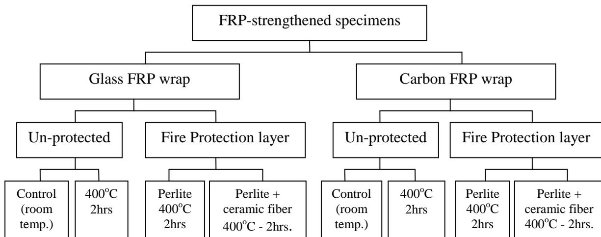
Fig.2 Experimental Program for FRP strengthened (confined) specimens
