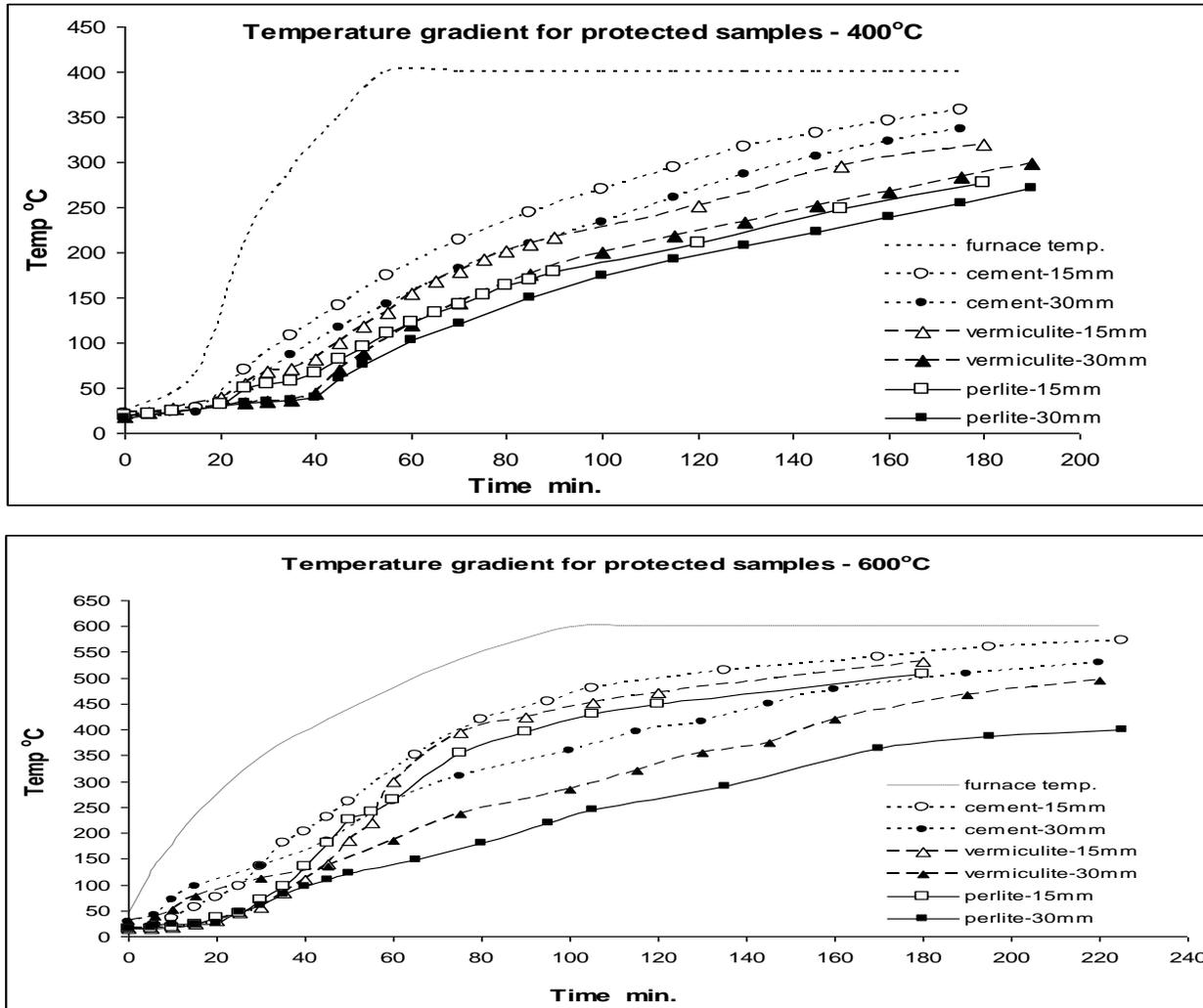
Fig.8: Temperature profile in protected unstrengthened specimens
