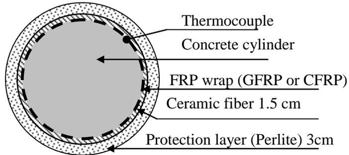
Fig.3 : Scheme of strengthening and protection layers applied to concrete cylinders.
