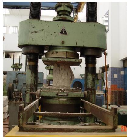
Fig.6: Experimental test set-up for testing the concrete cylinders.
