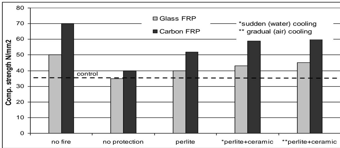
Fig 13: Effect of protection material on ultimate capacity of wrapped concrete specimens
