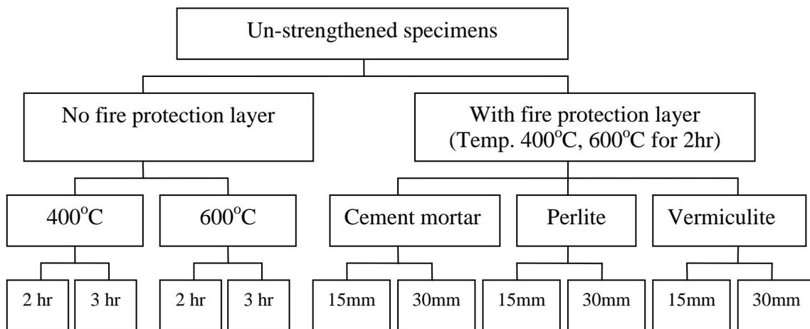
Fig.1 Experimental Program for unstrengthened specimens
