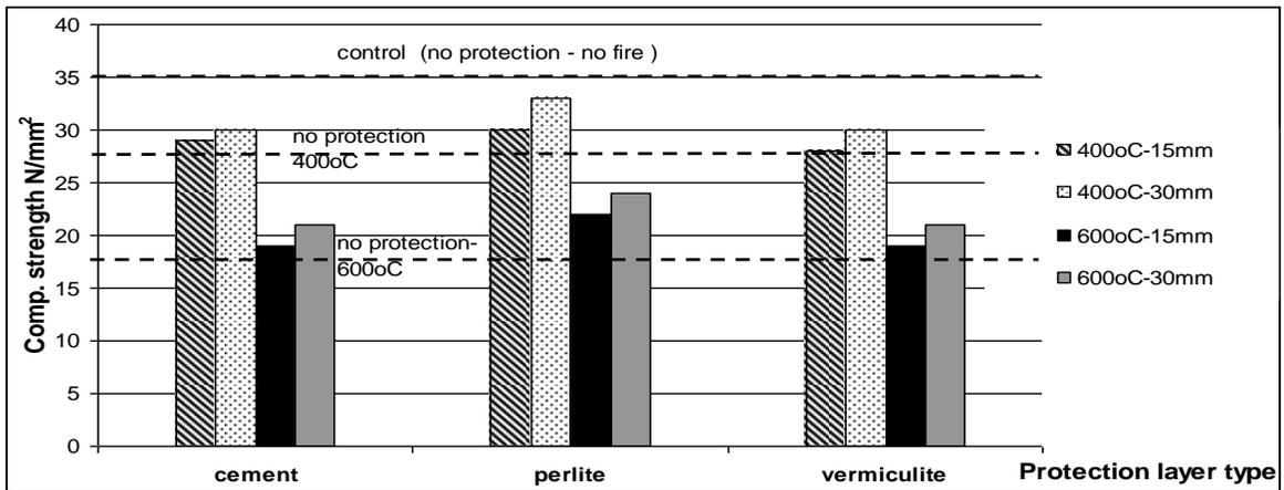
Fig 9: Effect of protection material and layer thickness on concrete strength
