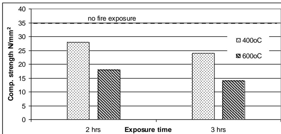
Fig 7: Effect of fire exposure on ultimate capacity of unprotected concrete specimens
