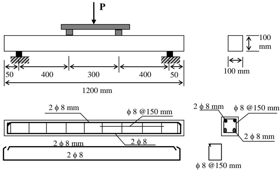
**Figure 1. Dimensions and reinforcement of tested beams.**
