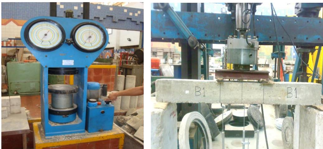
**Figure 4: Compression machine for testing cubes and 4-point bending test for beams**
