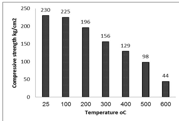
**Figure 5: Compressive strength of unprotected cubes after exposure to elevated temperatures.**
