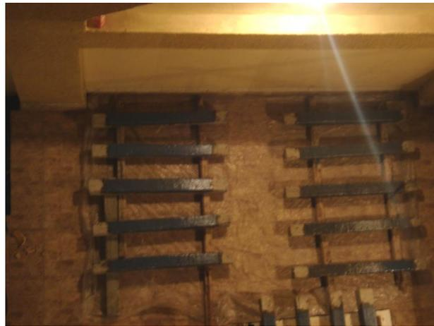
**Figure 2: RC beams strengthened by FRP**
