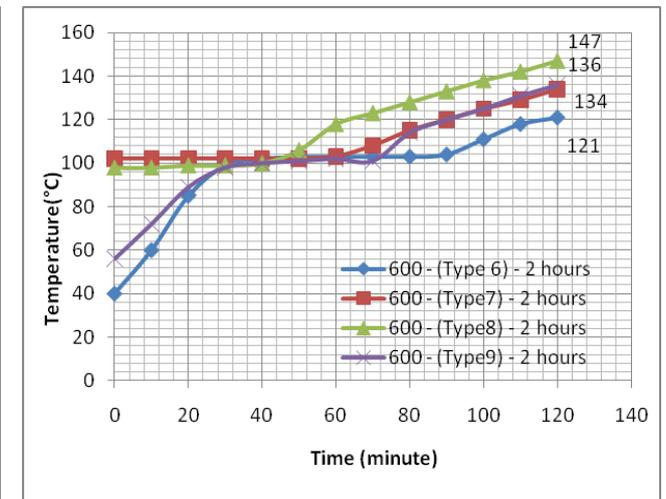
**Figure 6: Temperature measured under coatings exposed to 600°C for 2 hours.**
