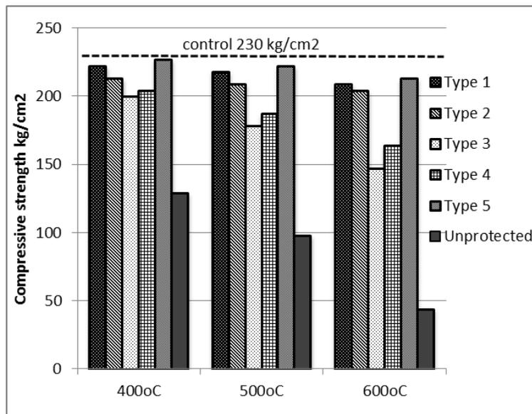
**Figure 7: Compressive strength for protected cubes with coating types 1-5 when exposed to 400, 500 and 600°C 2 hours.**
