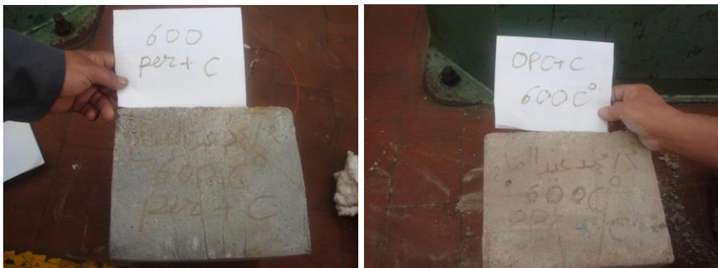
**Figure 8: Concrete cube with protection type(6) and type(8) after 2-hour exposure to 600°C.**
