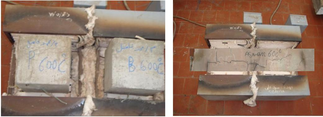
**Figure 3: Installation of concrete cubes and beams in the electric furnace.**
