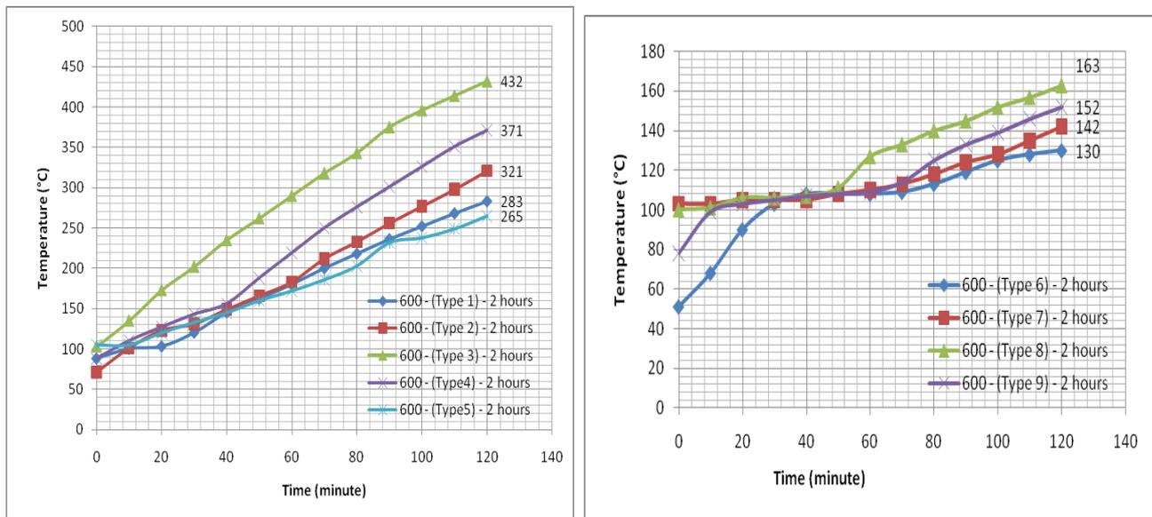
**Figure 9: Temperature measured under coating types 1-5 when exposed to 600°C for 2 hours.**
