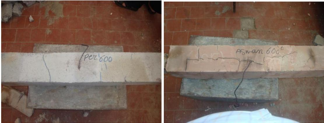
**Figure 10: FRP-strengthened RC beams protected using type 1 and 4 after exposure to 600°C.**
