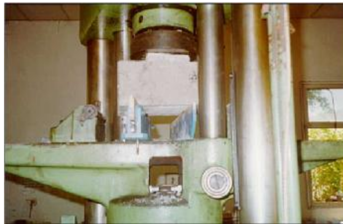
Fig. 7 Test of column head connection subject to shear loads
