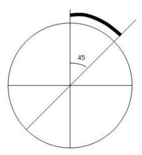
We know that there are 360 degrees in a circle. First we see that a circle is symmetrical about the x axis, so only the first 180 degrees need to be calculated. Next, we see that it's also symmetrical about the y axis, so now we only need to calculate the first 90 degrees. Finally, we see that the circle is also symmetrical about the 45 degree diagonal axis, so we only need to calculate the first 45 degrees.
