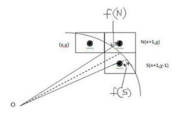
As can be easily intercepted, the continuous arc of the circle can not be plotted on a raster display device, but has to be approximated by choosing the pixels to be highlighted. At any point (x,y), we have two choices – to choose the pixel on east of it, i.e. N(x+1,y) or the south-east pixel S(x+1,y-1). To choose the pixel, we determine the errors involved with both S(x+1,y-1) and S(
