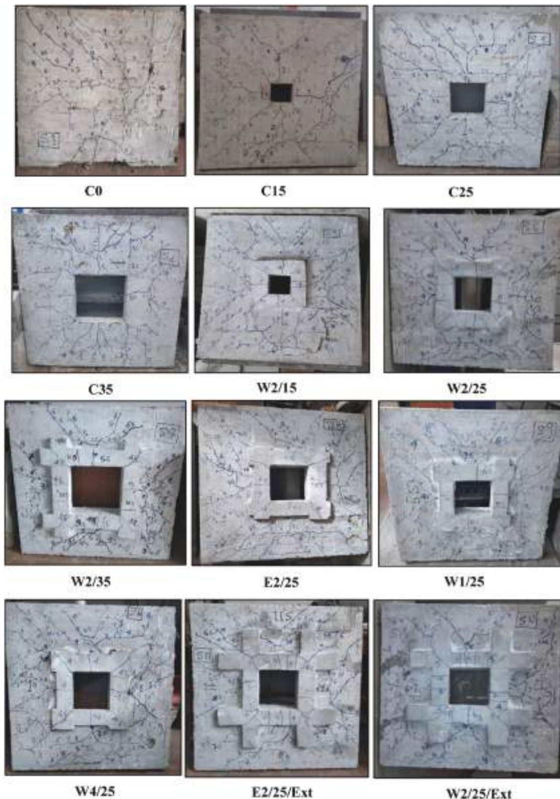
Fig.8. Crack pattern for the tested slabs (bottom faces).
