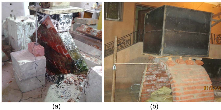
Fig. 5. Test setup for a) wallets and b) vaults.
