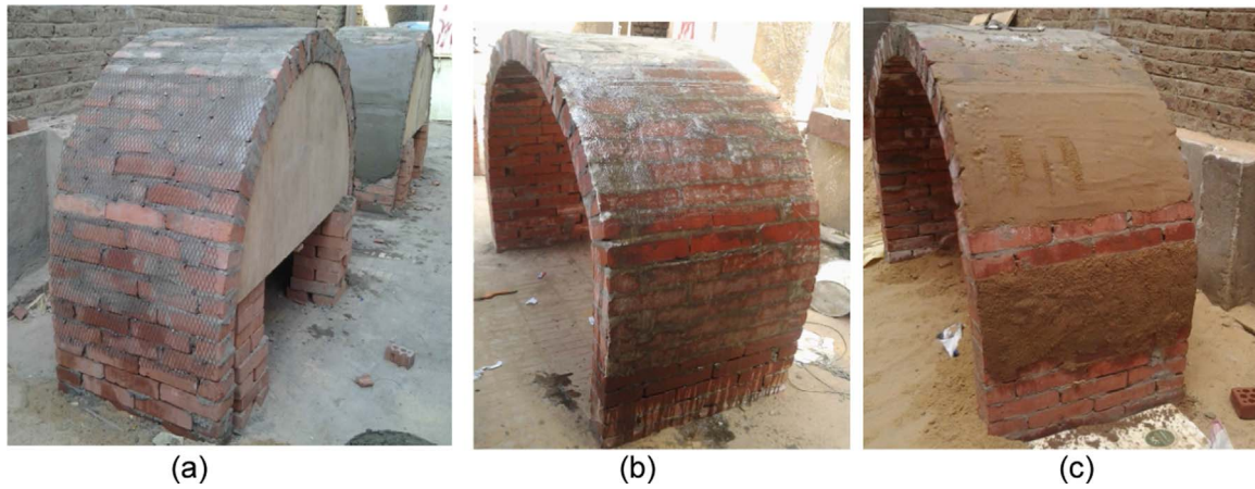
Fig. 4. Vaults after strengthening by a) ferro-cement wire mesh, b) GFRP sheets c) polyester mortar.
