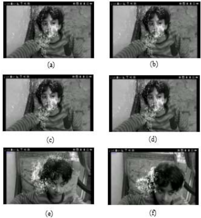
Fig. 6. System results using optical flow based on fast corner method (a) shows the first frame when detecting the face, and run the tracker, (b),(c), and (d) show the result of the tracker on some frames, (e), and (f) show false positive, and false negative.
