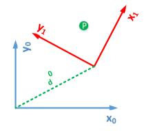
For composite homogeneous transformation, the rule for **pre** and **post** multiply is valid as rotation.
