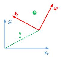
To use HTs in computing coordinates of point p, we need to extend the vectors of a point by one coordinate:
