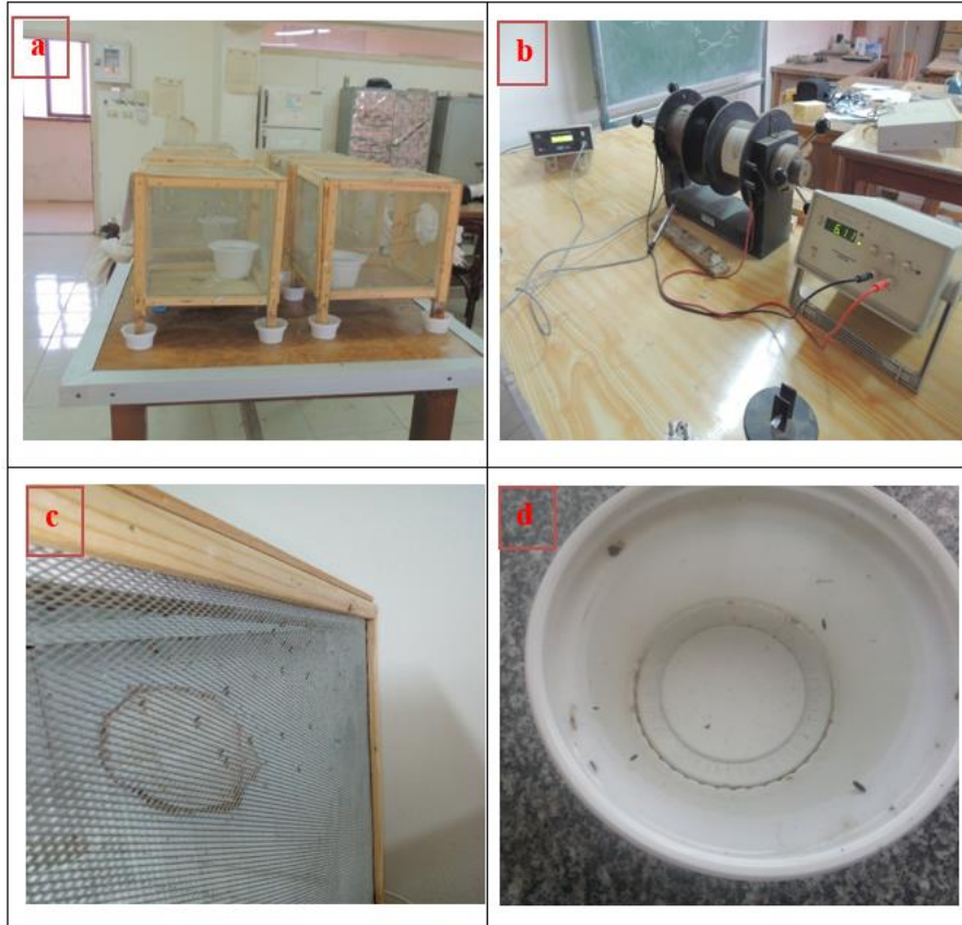
Fig. 1: Experimental aspects of the effect of the magnetic field on mosquito immature stages. Mosquito rearing (a), SMF exposing facility (b), blood-feeding (c), and hatchability (d).
