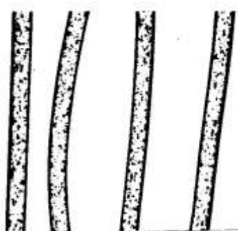
Figure 13: Photomicrograph of regular polyester fiber longitudinal view
