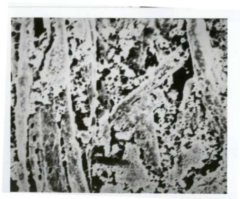
Figure 27: Photomicrograph of Azhar paper 1000 x
