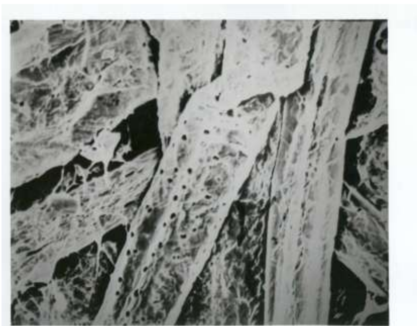
Figure 30: Photomicrograph of Edfo paper 1000 x
