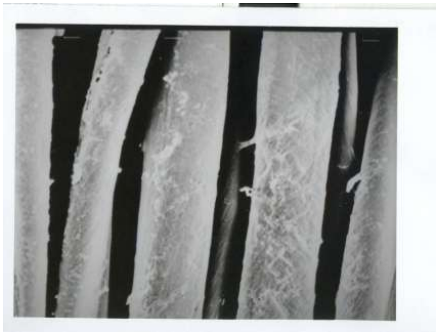
Figure 49: Photomicrograph of cotton 1500x
