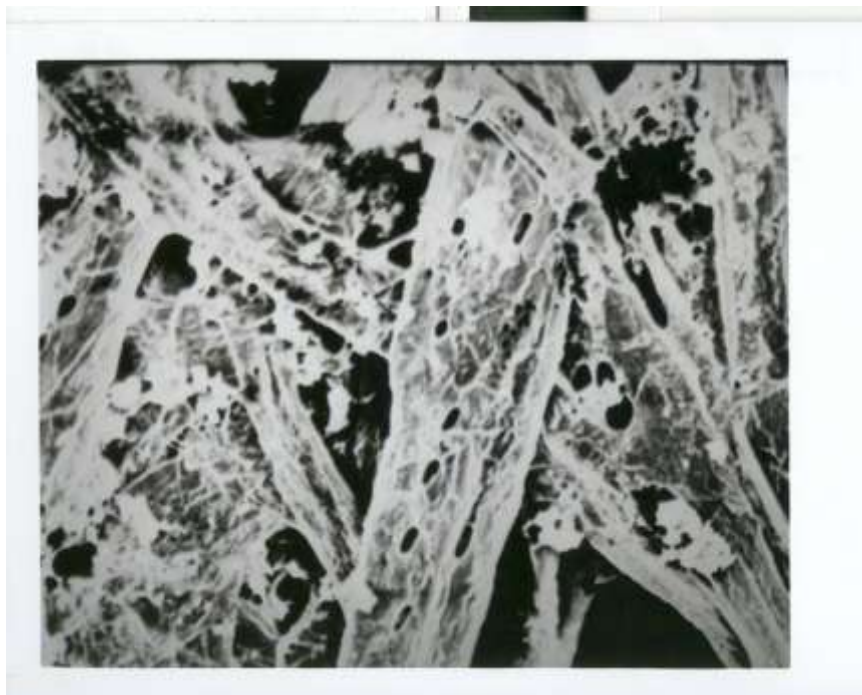
Figure 28: Photomicrograph of Xerox paper 1000x
