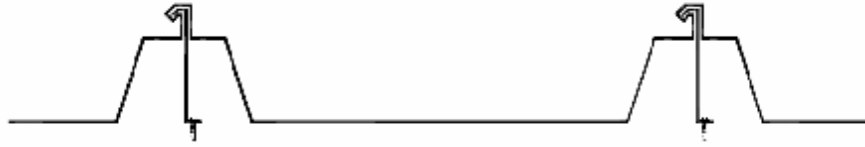
Figure 1.3: Profile of Standing Seam Roof Panel (Stolarczyk et al [42])
