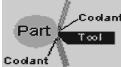
Figure (10): For heavy cutting, it is advisable to have cutting fluid directed at the top and bottom of the cutting area
