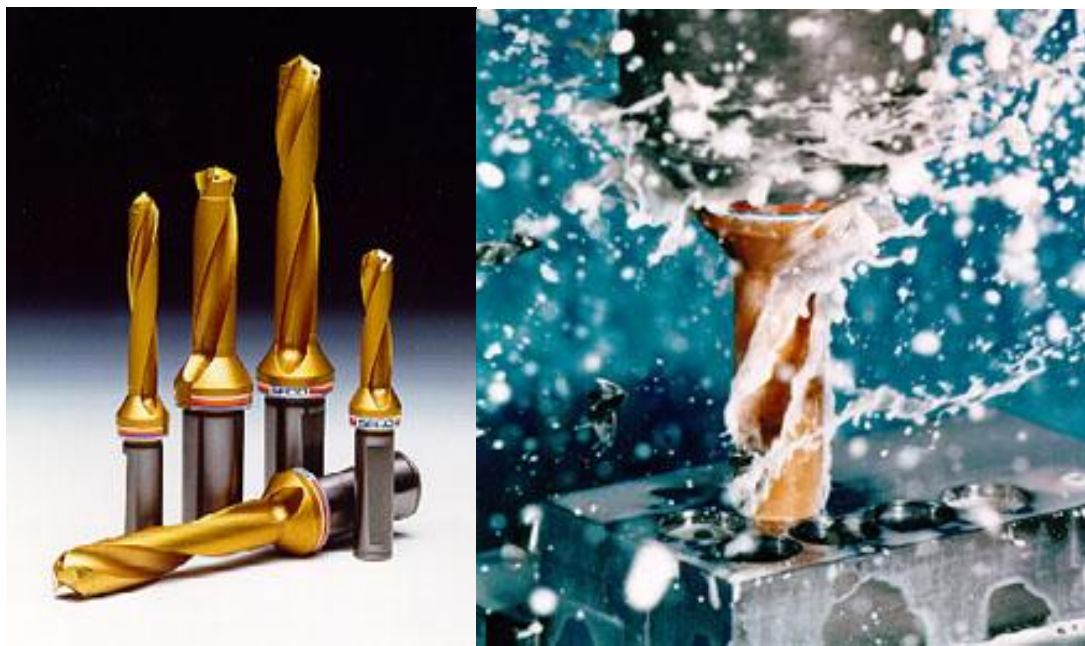
Figure (9): Oil hole drills will supply cutting fluid directly to the cutting edges of the drill.
