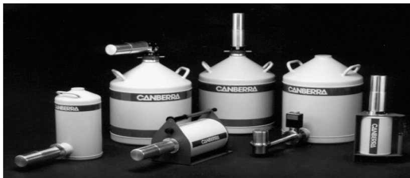
Figure (2.1); examples of HPGe detectors (Canberra)
