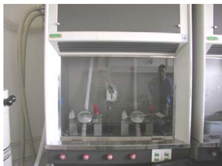
Figure (3.5); Fast transport pneumatic tubes (2 tubes available)
