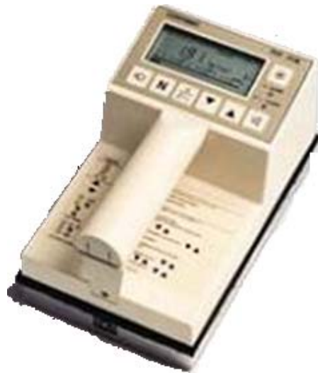
Figure (3.18): Large Area Contamination Monitors (LACSM)
