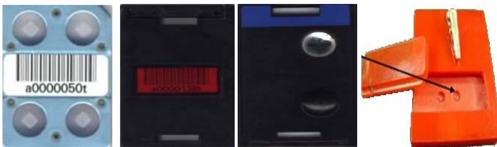
Fig (3.20); Portable Personnel Monitoring (TLD) chip and holders
