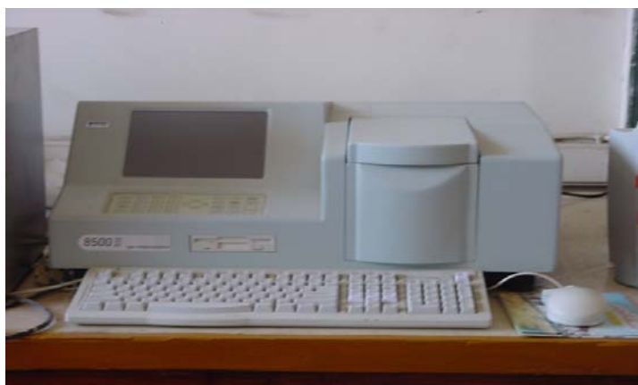
Figure (3.9); UV/VIS8500 Double-Beam spectrophotometer
