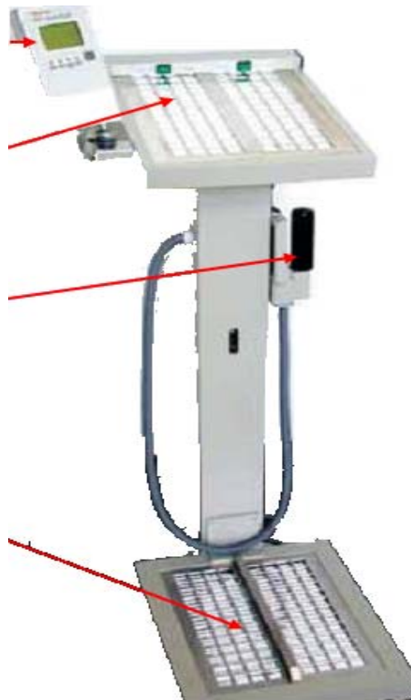
Figure (3.23); Hand, Feet and Clothes Monitors (HFCM)
