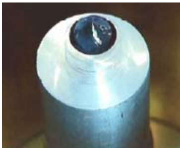
Fig.(4.1); The high-purity germanium crystal detector is housed in an evacuated container that is enclosed in a lead shield and the sample stone has been placed with its center of mass 7 cm above the detector.
