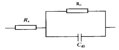
Figure (1.1); Electrical equivalent circuit model used to represent an electrochemical interface undergoing corrosion in the absence of diffusion control.  $R_p$  is the polarization resistance,  $C_{dl}$  is the double layer capacitance,  $R_p$  is the polarization resistance, and  $R_s$  is the solution resistance.
