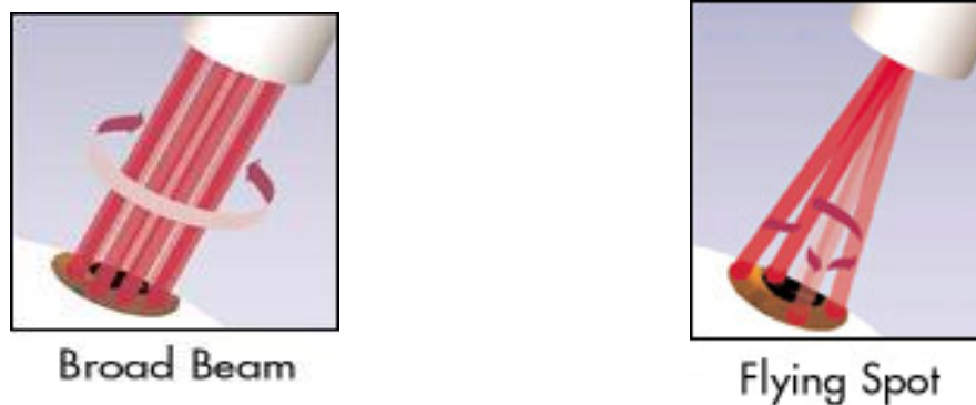
Figure (3.1) The broad beam and flying spot LASER
