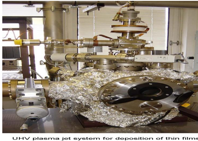
Fig 6-22 UHV Plasma jet system for deposition of thin films.
