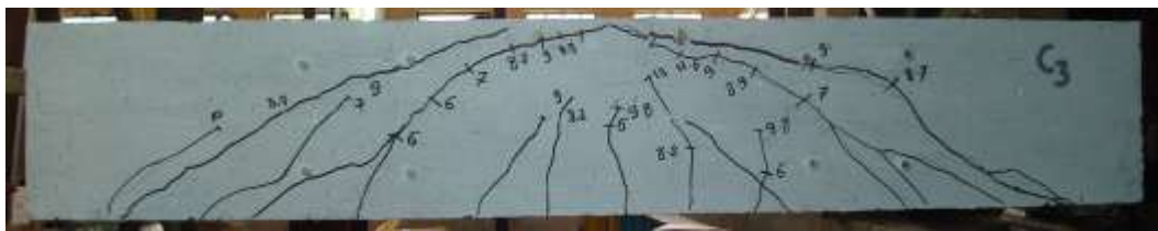
a) Beams A3, B3, and C3 with stirrups \rho_v = 0.24\%
