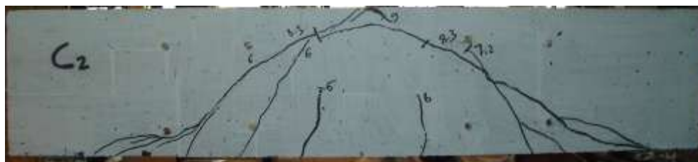
b) Beams A2, B2, and C2 without stirrups
