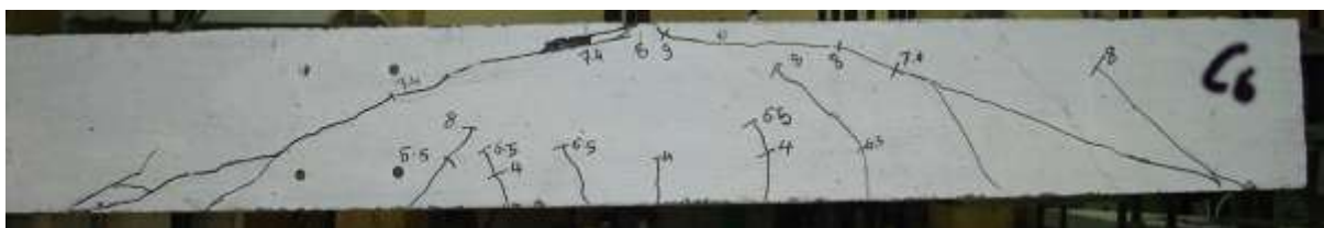
Figure (5-3) Crack Patterns of the Tested Beams with ( a/d = 4.5 )
