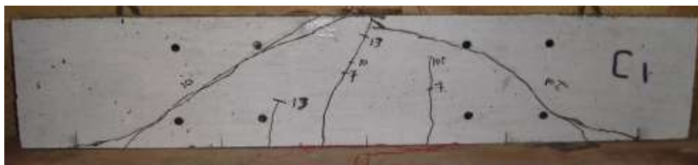
a) Beams A1, B1, and C1 with stirrups \rho_v = 0.24\%
