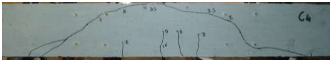
b) Beams A4, B4, and C4 without stirrups
