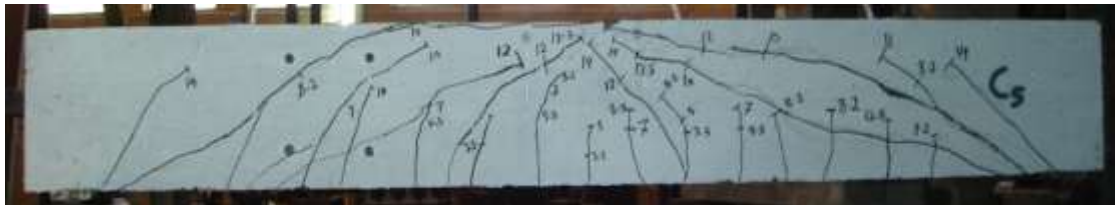
c) Beams A5, B5, and C5 with stirrups \rho_v = 0.48\%
