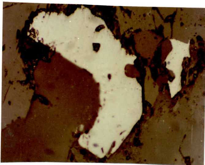
Fig. (3.23): Folded discrete ilmenite with irregular boundaries, biotite-free amphibolites, S 98 , RL, X 700 .
