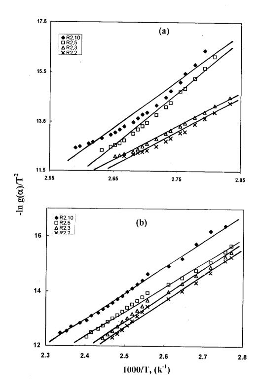
Fig.( III-A-14): Coats-Redfern method of analysis for dynamic dehydration of (a) zinc nicotinate and (b) cupper isonicotinate, assuming (R<sub>2</sub>) model.
