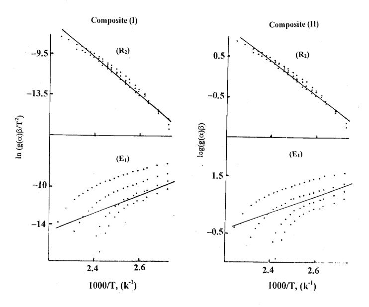
Fig.(III-A-6): Composite analysis of dynamic TG data of thermal dehydration of cobalt-nickel nicotinate, assuming (R<sub>2</sub>) and (E<sub>1</sub>) models.
