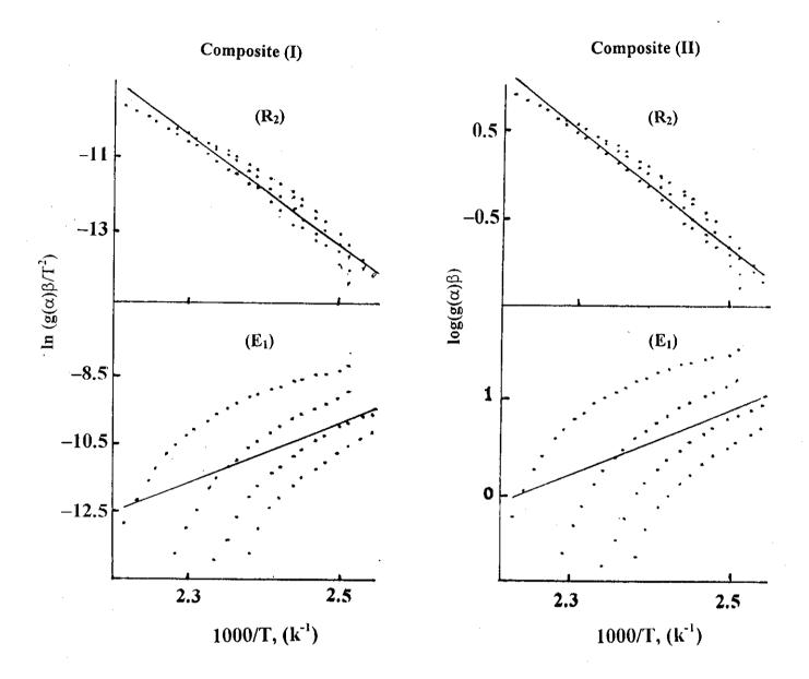
Fig.( III-A-8): Composite analysis of dynamic TG data of thermal dehydration of nickel isonicotinate, assuming  $(R_2)$  and  $(E_1)$  models.
