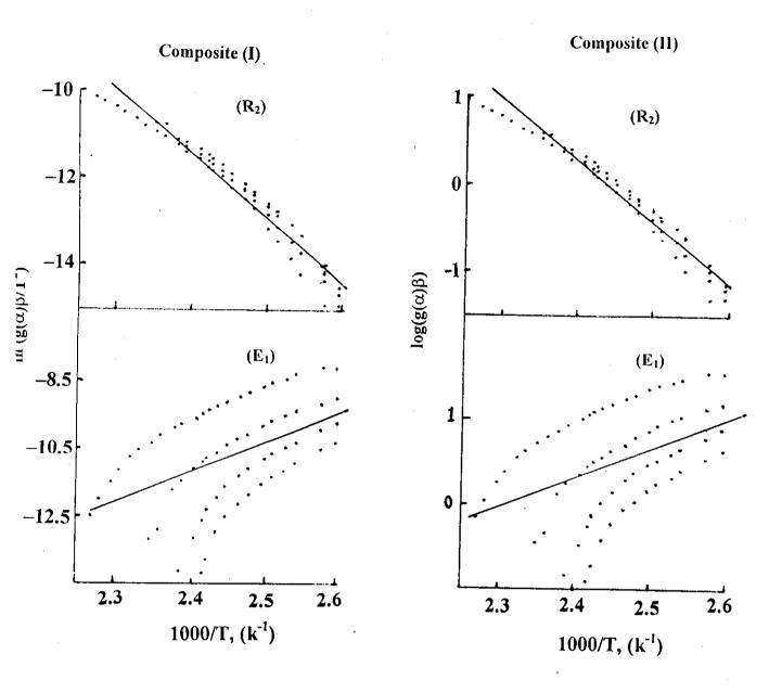
Fig.( III-A-9): Composite analysis of dynamic TG data of thermal dehydration of cobalt-nickel isonicotinate, assuming (R<sub>2</sub>) and (E<sub>1</sub>) models.
