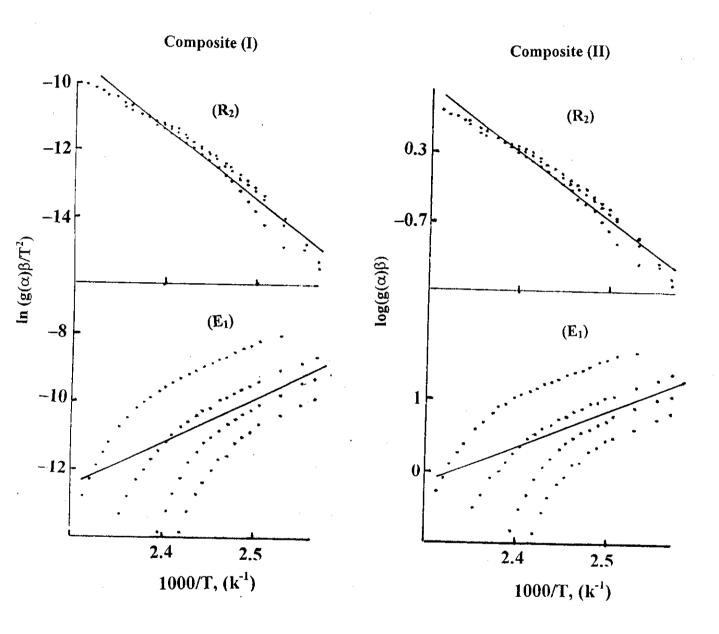
Fig.( III-A-4): Composite analysis of dynamic TG data of thermal dehydration of cobalt nicotinate, assuming (R<sub>2</sub>) and (E<sub>1</sub>) models.
