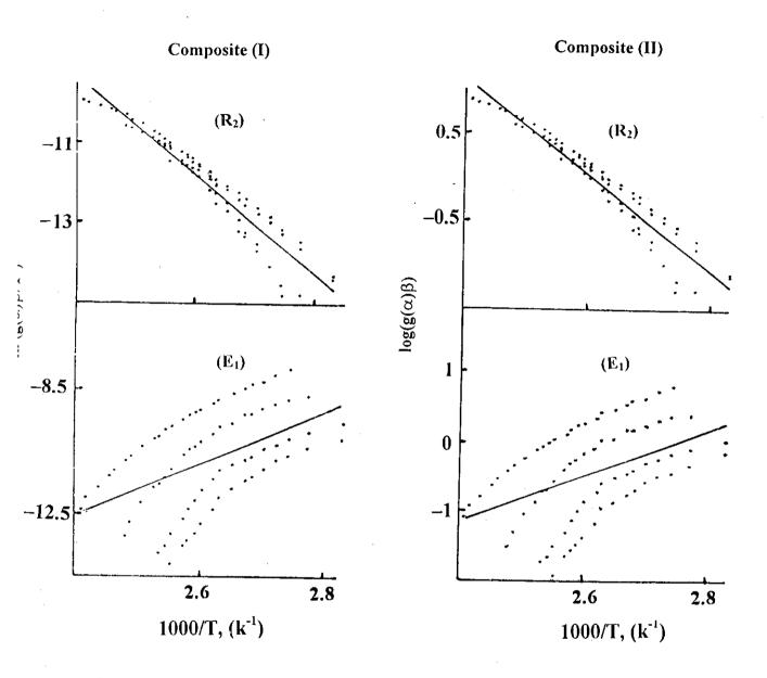
Fig.(III-A-11): Composite analysis of dynamic TG data of thermal dehydration of cupper isonicotinate, assuming  $(R_2)$  and  $(E_1)$  models.
