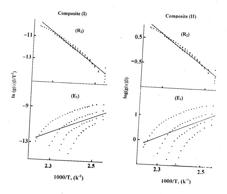
Fig.( III-A-5): Composite analysis of dynamic TG data of thermal dehydration of nickel nicotinate, assuming (R<sub>2</sub>) and (E<sub>1</sub>) models.
