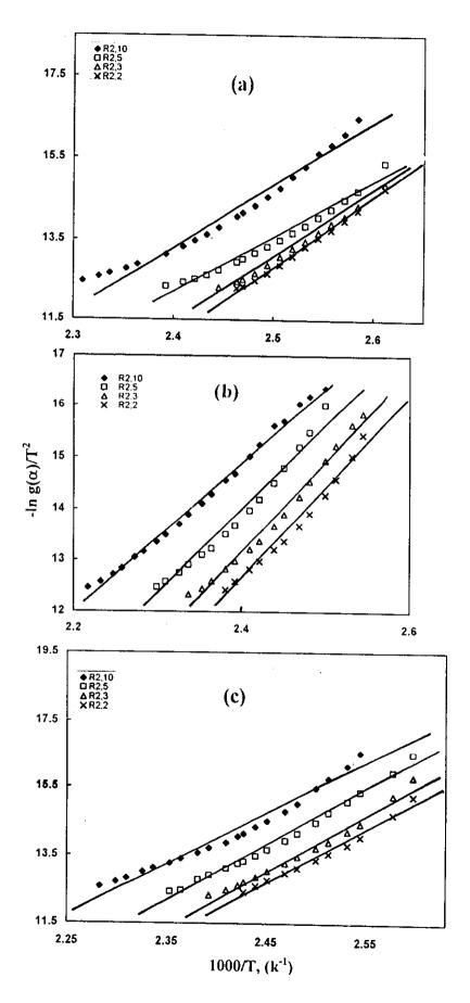
Fig.( III-A-13): Coats-Redfern method of analysis for dynamic dehydration of (a) cobalt isonicotinate, (b) nickel isonicotinate and (c) cobalt-nickel isonicotinate, assuming (R<sub>2</sub>) model.
