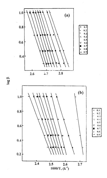
Fig.( III-A-17): Ozawa method of analysis for thermal dehydration of (a) zinc nicotinate and (b) cupper isonicotinate
