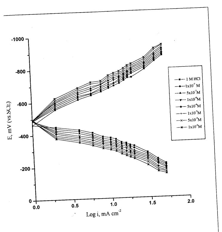
Fig.(3.24): Galvanostatic polarization curves for C-steel in 1 M HCl in the absence and presence of different concentrations of inhibitor (II-b)
