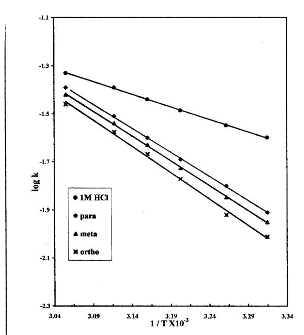
Fig (3.43): log K- 1/T curves for carbon steel dissolution in 1 M HCl in the absence and presence of 10<sup>-6</sup> M of inhibitor (IV-c)
