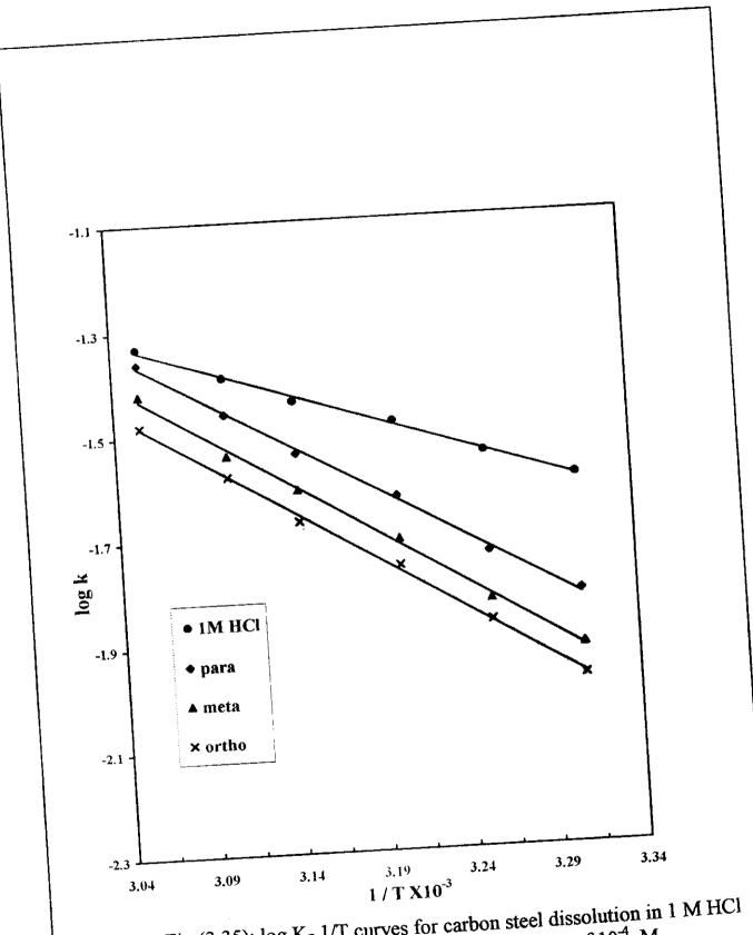
Fig (3.35): log K- 1/T curves for carbon steel dissolution in 1 M HCl in the absence and presence of 10<sup>-4</sup> M of inhibitor (II-a)
