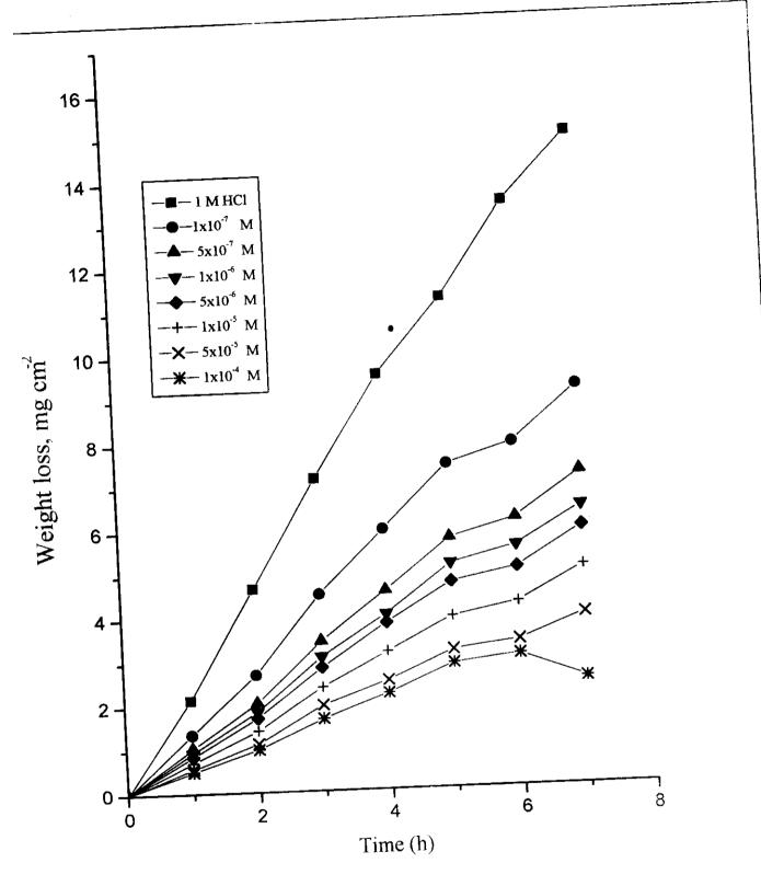
Fig.(3.12): Weight loss-time curves for C-steel dissolution in 1M HCl in The absence and presence of different concentrations of inhibitor (IV-c)
