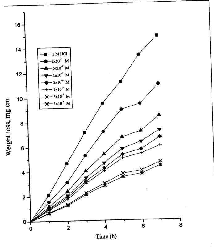
Fig. (3.5): Weight loss-time curves for C-steel dissolution in 1 M HCl in The absence and presence of different concentrations of inhibitor (II-b)
