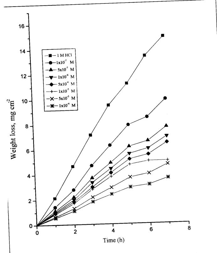
Fig. (3.7): Weight loss-time curves for C-steel dissolution in 1 M HCl in The absence and presence of different concentrations of inhibitor (III-a)
