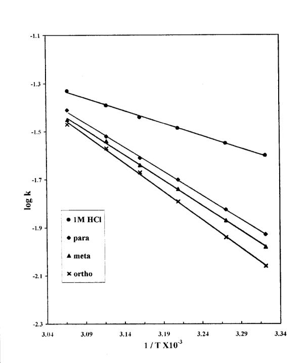
Fig (3.42): log K- 1/T curves for carbon steel dissolution in 1 M HCl in the absence and presence of 10<sup>-5</sup> M of inhibitor (IV-b)
