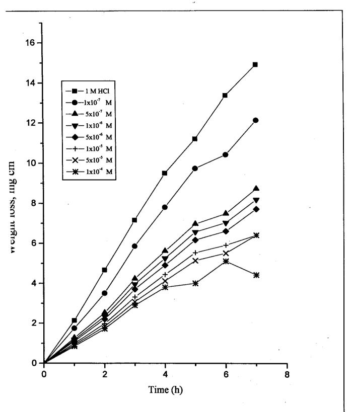
Fig. (3.9): Weight loss-time curves for C-steel dissolution in 1 M HCl in The absence and presence of different concentrations of inhibitor (III-c)
