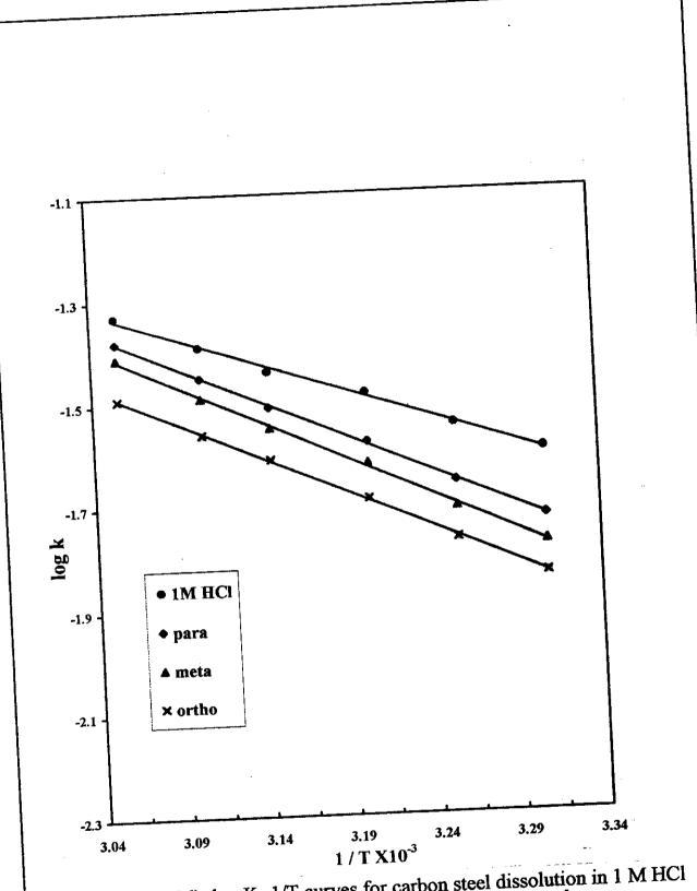
Fig (3.36): log K- 1/T curves for carbon steel dissolution in 1 M HCl in the absence and presence of 10<sup>-5</sup> M of inhibitor (II-b)
