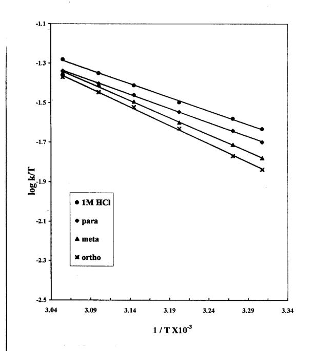
Fig (3.45): log K/T- 1/T curves for carbon steel dissolution in 1 M HCl in the absence and presence of 1x 10<sup>-4</sup> M of inhibitor (II)
