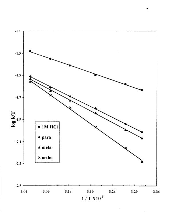
Fig (3.47): log K/T- 1/T curves for carbon steel dissolution in 1 M HCl in the absence and presence of 1x 10<sup>-4</sup> M of inhibitor (IV)
