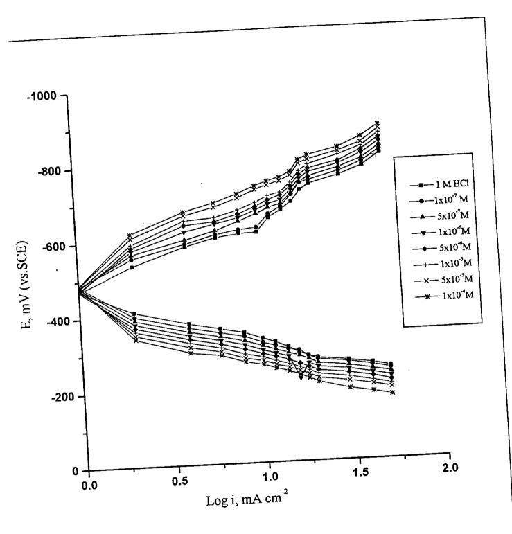
Fig.(3.23): Galvanostatic polarization curves for C-steel in 1 M HCl in the absence and presence of different concentrations of inhibitor (II-a)
