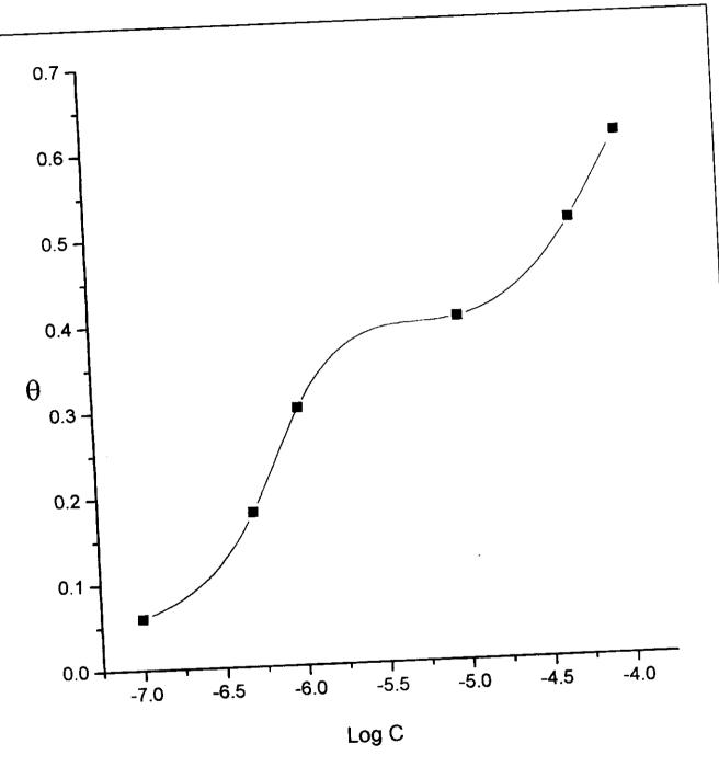
Fig. (3.13): Dependence of  $\theta$  on the logarithm of inhibitor (I) concentrations
