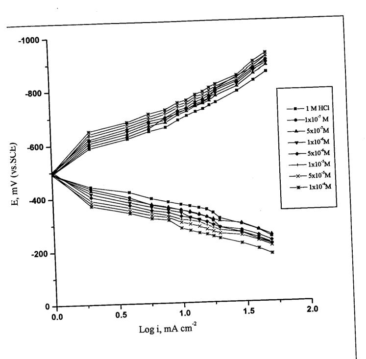
Fig.(3.26): Galvanostatic polarization curves for C-steel in 1 M HCl in the absence and presence of different concentrations of inhibitor (III-a)
