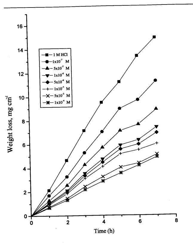
Fig. (3.6): Weight loss-time curves for C-steel dissolution in 1 M HCl in The absence and presence of different concentrations of inhibitor (II-c)
