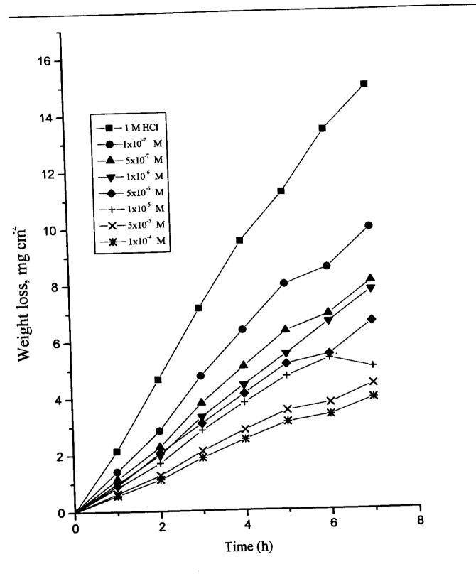
Fig. (3.4): Weight loss-time curves for C-steel dissolution in 1 M HCl in The absence and presence of different concentrations of inhibitor (II-a)
