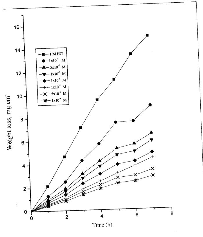
Fig. (3.11): Weight loss-time curves for C-steel dissolution in 1 M HCl in The absence and presence of different concentrations of inhibitor (IV-b)
