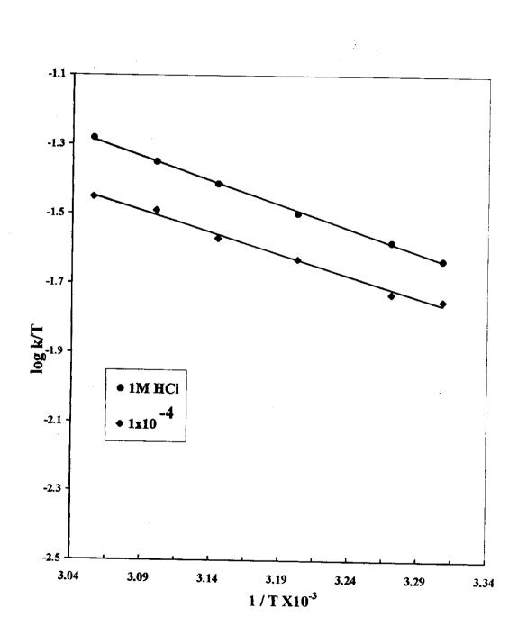
Fig (3.44): log K/T- 1/T curves for carbon steel dissolution in 1 M HCl in the absence and presence of 1x 10<sup>-4</sup> M of inhibitor (I)
