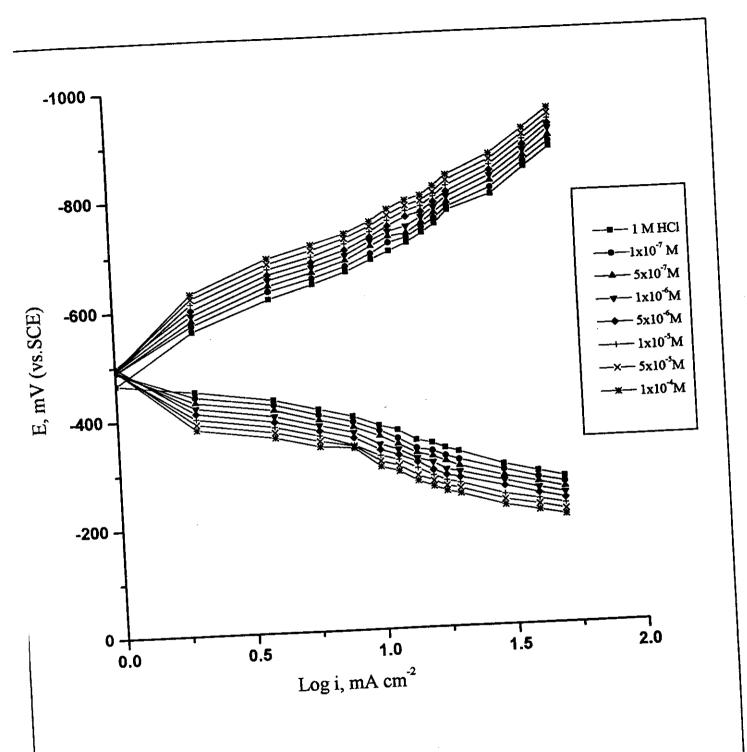
Fig.(3.25): Galvanostatic polarization curves for C-steel in 1 M HCl in the absence and presence of different concentrations of inhibitor (II-c)
