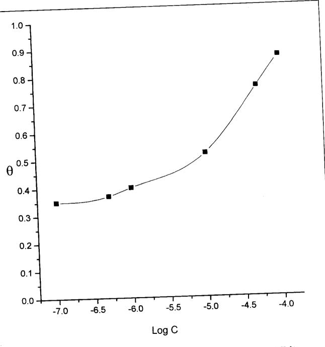
Fig. (3.21): Dependence of  $\theta$  on the logarithm of inhibitor (IV-b) concentrations
