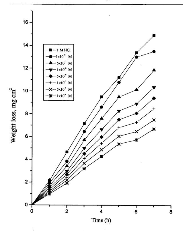
Fig. (3.1): Weight loss-time curves for C-steel dissolution in 1 M HCl in The absence and presence of different concentrations of inhibitor (I)
