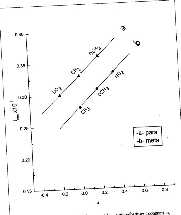
Fig. (3.33): Variation of corrosion curent  $I_{corr}$ , with substituent constant,  $\sigma$ , of the substituent group in (a)para and (b) meta position with respect of the azo group of indole derivatives
