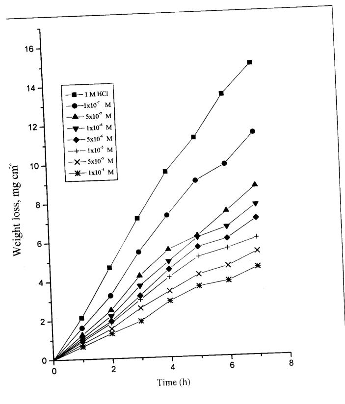
Fig. (3.8): Weight loss-time curves for C-steel dissolution in 1 M HCl in The absence and presence of different concentrations of inhibitor (III-b)
