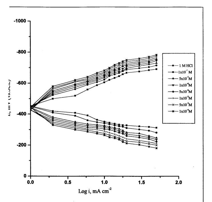
Fig.(3.2): Galvanostatic polarization curves for C-steel in 1 M HCl in the absence and presence of different concentrations of inhibitor (I)
