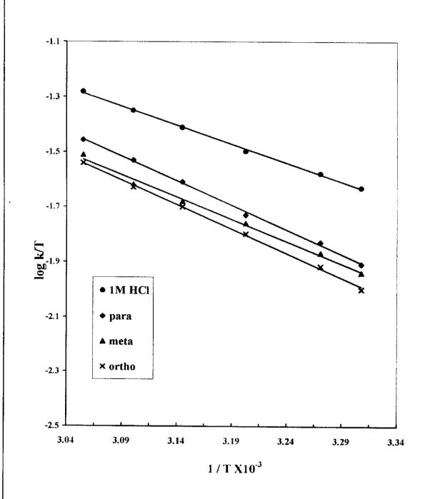
Fig (3.46): log K/T- 1/T curves for carbon steel dissolution in 1 M HCl in the absence and presence of 1x 10<sup>-4</sup> M of inhibitor (III)
