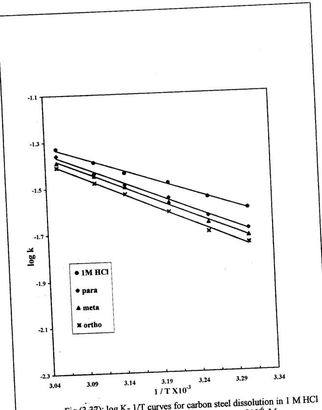
Fig (3.37): log K- 1/T curves for carbon steel dissolution in 1 M HCl in the absence and presence of 10<sup>-6</sup> M of inhibitor (II-c)
