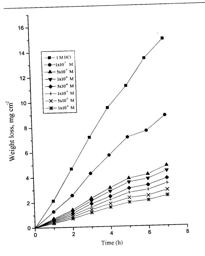
Fig. (3.10): Weight loss-time curves for C-steel dissolution in 1 M HCl in The absence and presence of different concentrations of inhibitor (IV-a)
