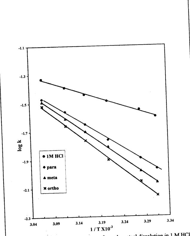
Fig (3.41): log K- 1/T curves for carbon steel dissolution in 1 M HCl in the absence and presence of 10<sup>-4</sup> M of inhibitor (IV-a)
