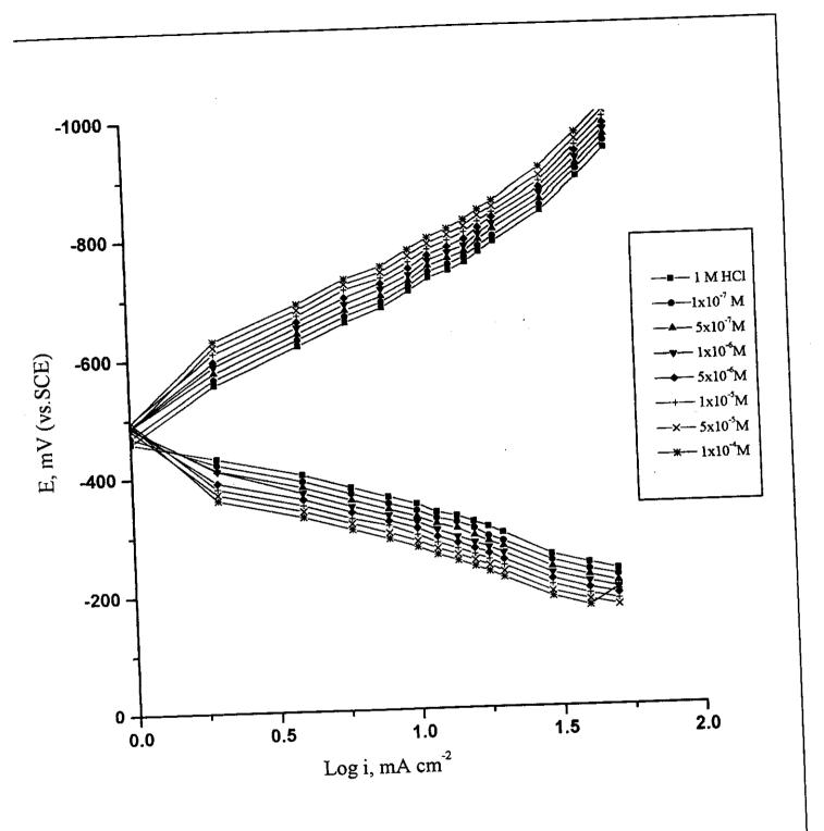
Fig.(3.28): Galvanostatic polarization curves for C-steel in 1 M HCl in the absence and presence of different concentrations of inhibitor (III-c)
