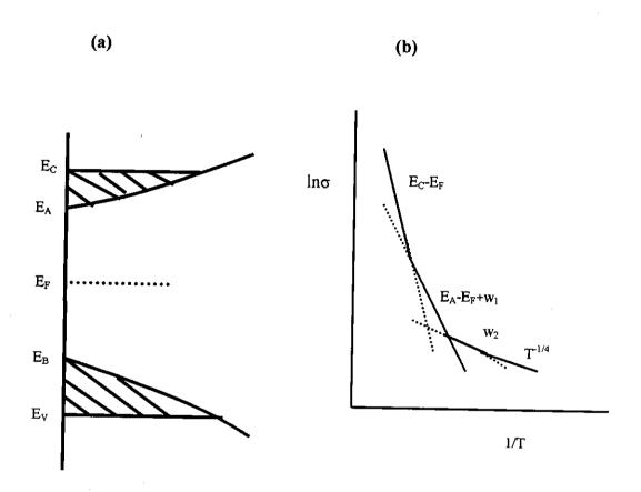
Fig. (2-1) (a)A real gap in the density of states, suggested here as a continues random network with defects. (b) Illustration of the temperature dependence of conductivity,  $\sigma = e \int N(E) \mu(E) F(E) dE$ .
