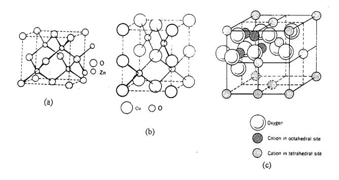
Fig.(I-1): The structure of (a) ZnO, (b) CuO and (c) Co<sub>3</sub>O<sub>4</sub>.
