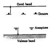
Fig(II-1): Energy levels in an insulator or semiconductor.
