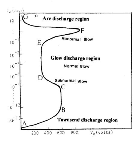
Fig. (1) The I-V characteristic curve of the electrical discharge.
