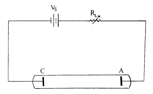
Fig.(2) Circuit used to Establish Glow discharge .-
