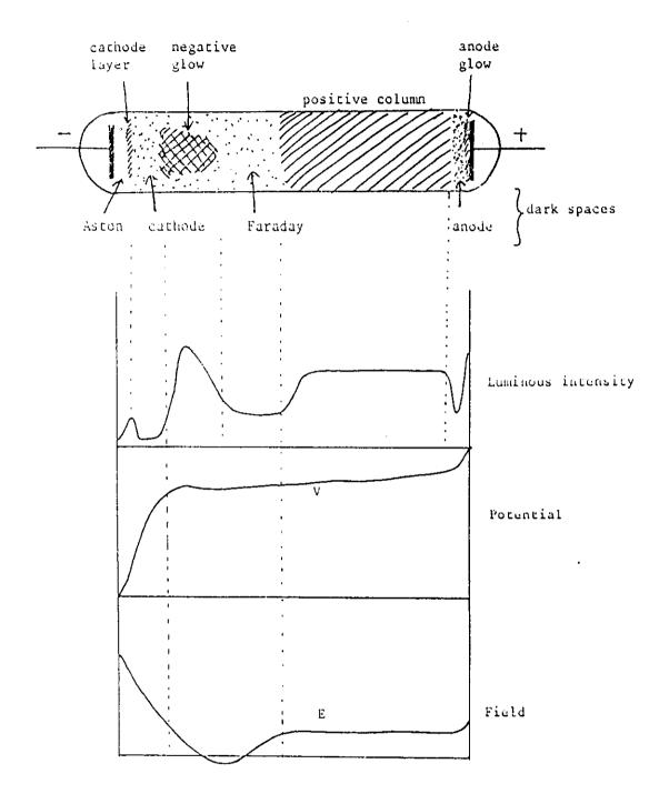
Fig. (3) The regions, luminous intensity, potential and electric field distributions of the glow discharge.
